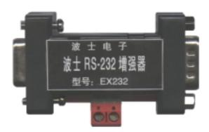
EX232 has an DB-9 /DB-9 connector shape. The female DB-9 side of EX232 is insertted to PC's RS-232 socket. The male DB-9 side of EX232 is a new RS-232 port which can communicate up to 500~1000meters. PC's RS-232 socket(DB-9 female):
